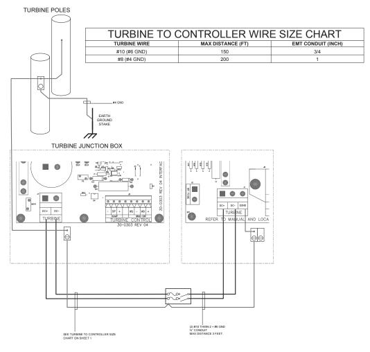
Figure 2.6 Turbine Circuit Diagram
